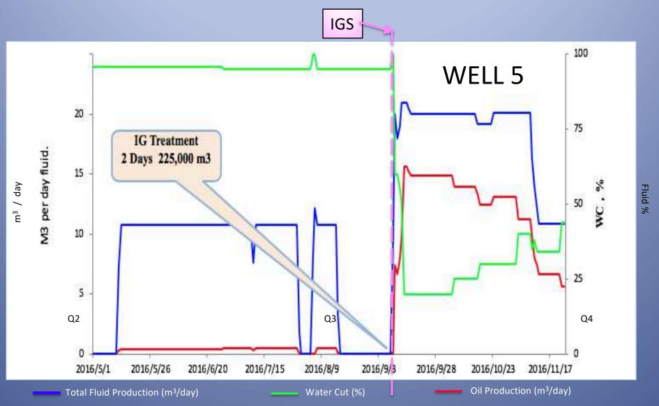
Production before IGS was 3.5 BOPD (95% Water Cut) After IGS was 98 BOPD with 25% Water Cut. Post IGS incremental Oil 5,900 Bbls in 70 days
