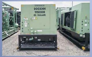
5 x Sullair 11500 SCFM Compressors running a 70% load
