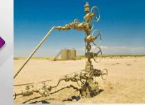
Immiscible Gas Blend and Connected to Wellhead
